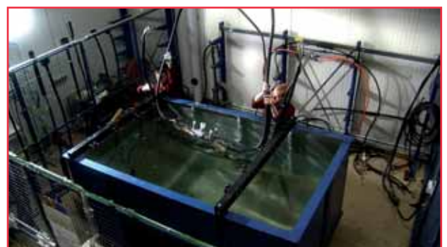
Cable sets in fatigue testing
