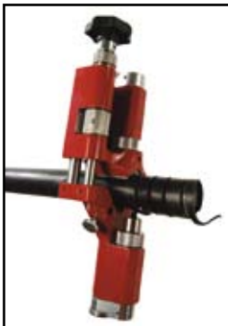
Incise and remove the External sheath
