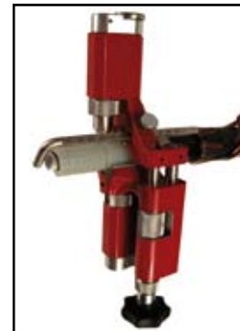
Incise and remove the external sheath
